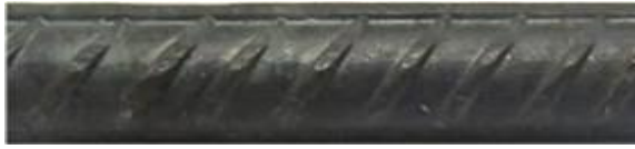
(a) Uncoated steel rebar
